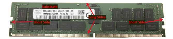
1(c): notches being formed on the short sides for being secured by the locking device; and;—SK Hynix makes, uses, sells, and/or offers to sell a memory module structure having notches formed on the short sides and the notches are operable to be secured by a locking device.
