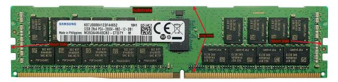
1(c): notches being formed on the short sides for being secured by the locking device; and;—Samsung makes, uses, sells, and/or offers to sell a memory module structure having notches formed on the short sides and the notches are operable to be secured by a locking device.
