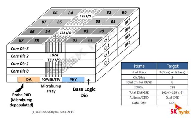
(See Ex. 19). Each "die" is a separate semiconductor chip, connected by TSVs and organized into vaults, e.g., B0, B1, B2, B3.
