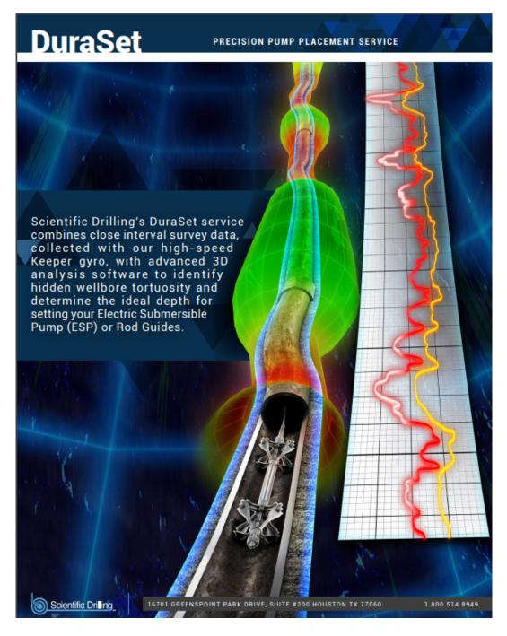
23. SDI's DuraSet obtains and uses close interval gyro survey log data with a log data density at as close as one-foot intervals. Exhibit 6 (DuraSet brochure) at 2. The "[c]lose interval log data ensures small positional changes in the well are properly measured and accounted for."
