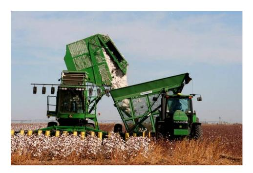
14. Next, the tractor would dump or spill the cotton from the boll buggy into a third machine called a "module builder."
