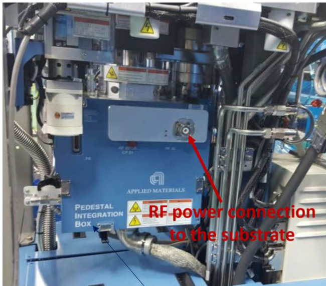
The Pedestal Integration Box (PIB) couples the RF bias power supply to the substrate (not shown) via the substrate area
