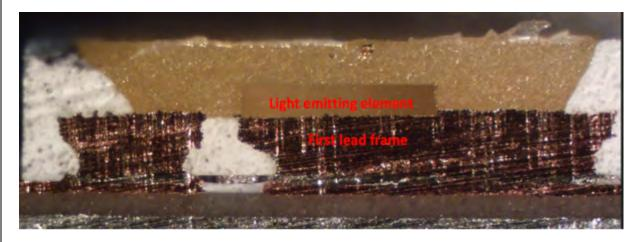
As another example, shown below is the cross-sectional view of the LED from the SpaceView Baby Monitor with an identification of a first lead frame on which the semiconductor light emitting element is mounted:
