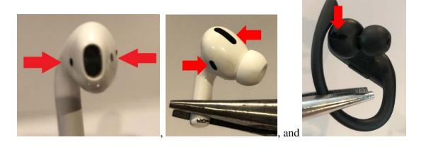
34. Claim 4 of the '320 patent covers the system of Claim 1 wherein the lid has a second magnet disposed within it. The Apple Infringing Products comprise the system of claim 1 (see above), wherein the lid of the switching device has a plurality of magnets disposed within it. For example (as noted by the below beads on the lids at left),
