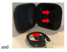
38. Claim 10 of the '320 patent covers the system of Claim 4 wherein the second or a third magnet is employed in the lid to actuate the electronic circuit. The Apple Infringing Products
