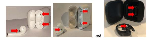
51. The Apple Infringing Products comprise the switching device (here the original charging case and/or wireless charging case) and the electronic device (here the earbud(s)) being configured to selectively couple to each other through a magnetic force, as noted in the above images.
