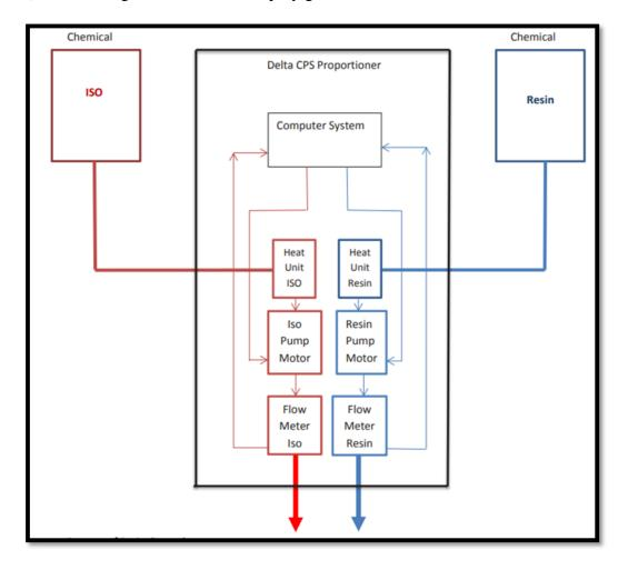
As seen in the above schematic, a flow meter near the pump output reads the amount of each chemical being released; this allows a primary pump to adjust the flow of the chemicals to ensure the desired ratio is consistently achieved at the point of spray application.
