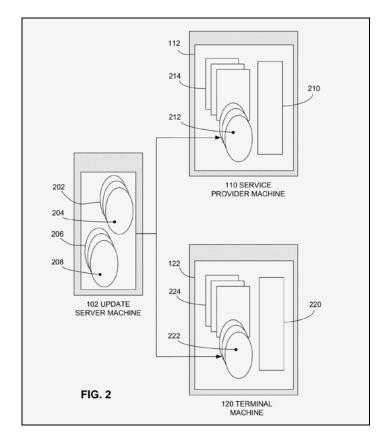
16. In like fashion, as shown in FIG. 2, the service provider machine runs an application having a very specific structure: namely, the provider application 112 comprises second computer-executable instructions 214, which can be directly executed on a processor, and second code 212, which must be translated before it can be executed on a processor. The provider application conducts the service provider's portion of the dialogue with the terminal machine.
