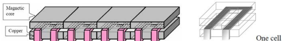
Figure 4.15 A scalable multi-phase surface mount coupling inductor structure proposed by Volterra in [77]
