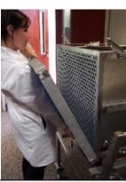
at least one opening in at least one of the plurality of panels to allow flow of the sterilization agent from an exterior of the cabinet directly to the interior sterilization area; The door has a plurality of openings to allow flow of the sterilization agent from an exterior of the POD cabinet directly to the interior sterilization area (Ex. G pg. 2)
