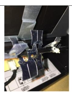
the paddle elements being located in the respective predetermined locations therefor to position the perimeter plane substantially perpendicular to the axis, for intermittently reflecting the light from said at least one light source from said at least one reflective surface to predetermined regions on the screen respectively as the flicker element rotates about the axis, to provide the images of flickering flames
