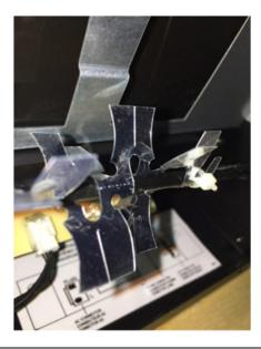
a plurality of paddle elements located in respective predetermined locations on the rod, each said paddle element comprising at least one body portion having at least one reflective surface
