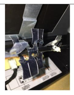
a plurality of paddle elements located in respective predetermined locations on the rod, each said paddle element comprising at least one body portion with at least one reflective surface thereon, said at least one reflective surface being formed to comprise a substantially planar region substantially defining a perimeter plane and a non-planar region;
