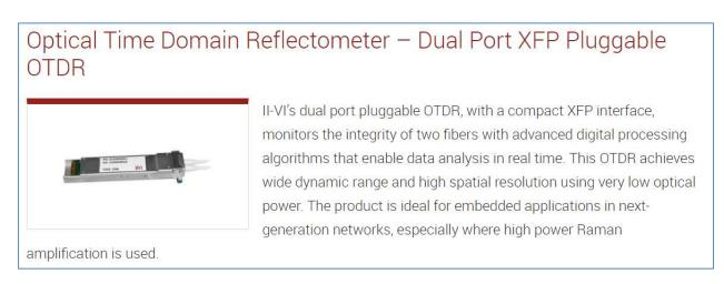
See <a href="https://optical.communications.ii-vi.com/roadms-wavelength-management/optical-time-domain-reflectometer-%E2%80%93-dual-port-xfp-pluggable-otdr">https://optical.communications.ii-vi.com/roadms-wavelength-management/optical-time-domain-reflectometer-%E2%80%93-dual-port-xfp-pluggable-otdr</a>.
