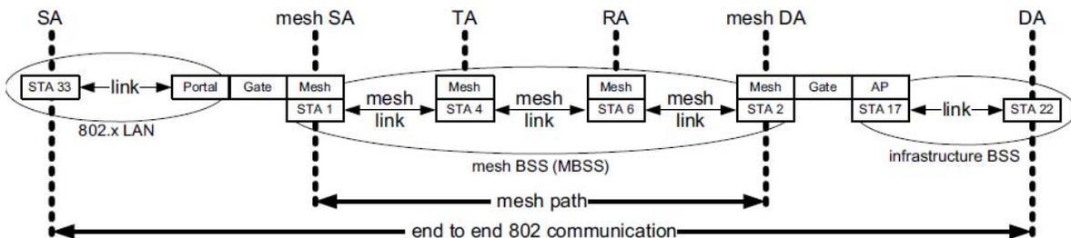
Figure 9-38—Example addressing for a Mesh Data frame
