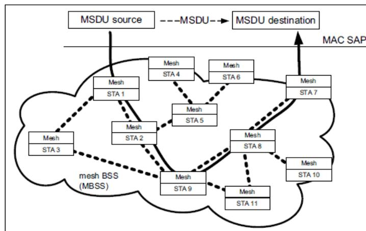
As shown below, while utilizing the active path selection protocol to determine the best path to a destination node, a hop which lies in route receives a path request PREQ with a forwarding information item, wherein basic forwarding information includes destination address, next-hop
