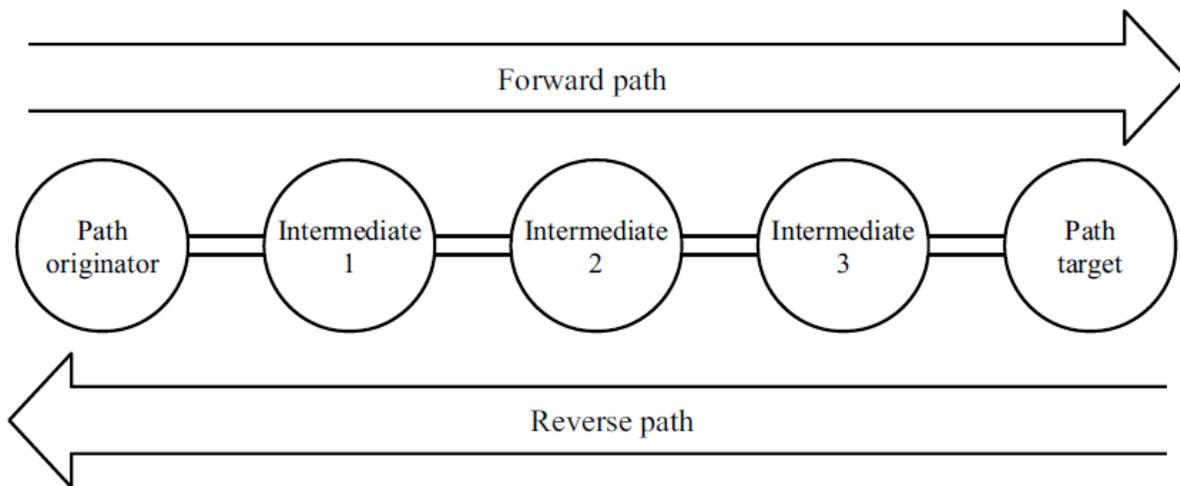
**forwarding information:** The forwarding information maintained by an originator mesh STA, an intermediate mesh STA, or a target mesh STA that allows the mesh STA to perform its path selection and forwarding functions.
