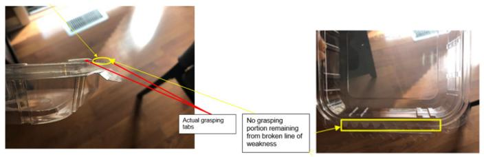
27. As seen above, when the line of weakness is severed, the remaining portion does not provide any section which could be used to facilitate removal.
