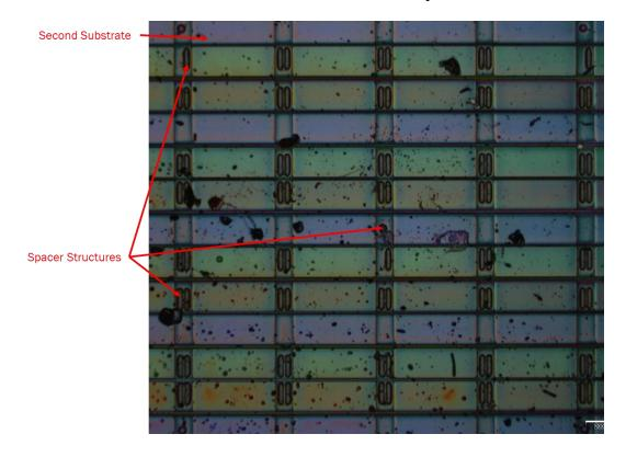
40. As shown in the analysis below, the spacer structure includes two types of spacers with one that is shorter than the other.
