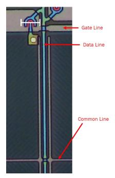
33. The Accused Panel has a data line intersecting the gate line with a gate insulating film between.
