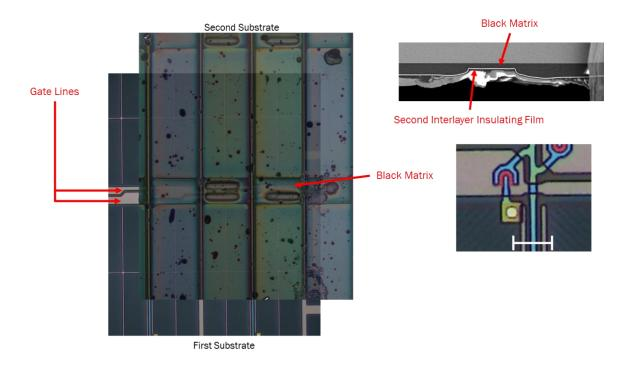
36. The Accused Panel shown below has a columnar spacer located above the gate line apart from the intersection of the gate and data lines.
