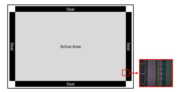
44. The Accused Panel shown below has a spacer in the seal to make a gap between the array substrate and the opposing substrate constant.
