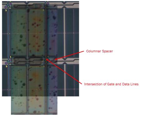
37. The Accused Panel also includes a second orientation film coating the second insulating film and the columnar spacer, as shown below.
