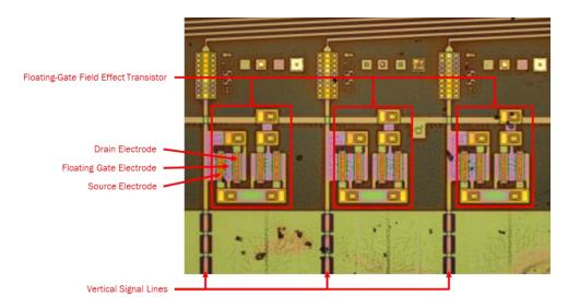
48. In the Accused Panel, the transistors respond to surge potentials on the vertical signal lines by turning on and establishing a low-impedance path to ground.
