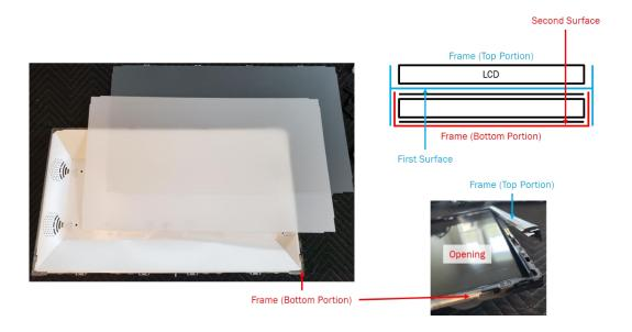
63. The optical unit has a conductive plate positioned in the opening of the frame, which has surfaces adjacent to the two frame surfaces (i.e., first and second surfaces), as shown and illustrated below.
