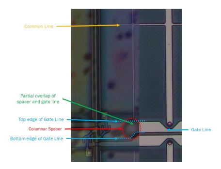
39. The Asserted Patents also cover Accused Panels, such as HKC TFT-LCD panel model no. PT320AT01-4, that include a substrate with a spacer structure.
