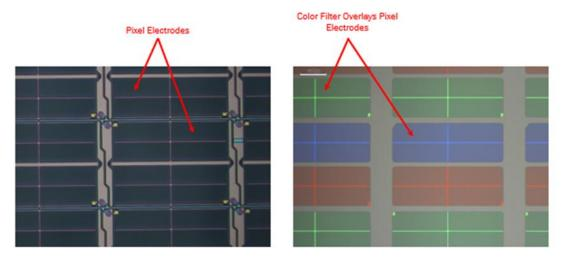
31. The Accused Panels have an active matrix type liquid crystal display device with two opposing insulating substrates and liquid crystal in-between, as illustrated below in reference to HKC TFT-LCD panel model no. PT320AT01-4.
