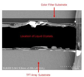
30. Each TFT acts as a switch that operates its respective individual pixel using the circuity lines. In that way, the pixels can be turned on and off to create an image on an LCD by allowing or preventing light to pass through. The individual pixels are more apparent when a color filter layer overlays the circuits as shown in the image below for the HKC TFT-LCD panel model no. PT320AT01-4.
