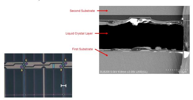
32. As shown below, the TFT-LCD Accused Panel contains a first substrate with a gate line, a common line parallel to the gate line.
