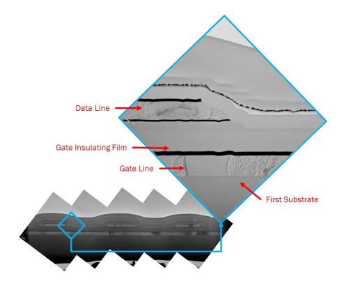
34. The Accused Panel also has a first interlayer film coating the data line and a first orientation film coating the first interlayer insulating film, as shown below.
