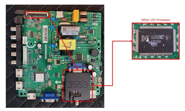
54. The Asserted Patents also cover Sceptre TVs and monitors that utilize an Mstar display controller, for example Mstar model nos. MSD3553NBCT-005X and MSD3553ZUC-005X are utilized in Sceptre model nos. E32 and H43 with HKC panel nos. PT320AT01-4 and PT430CT01-1, respectively. These Accused Panels have a clamping circuit for an LCD, as shown below in the MST703 LCD processor, which is expected to have features and components similar (or identical) to other as other MStar LCD processors.
