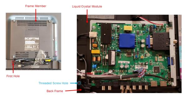
67. As shown below, there is a screw for attaching the frame member to the liquid crystal module from the back and through the hole in the frame member and the threaded screw hole in the back of the frame of the liquid crystal module.
