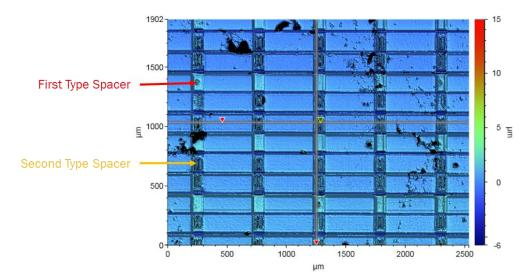
41. The first type spacer is over a red filter layer and the second type spacer is over a blue/green filter layer, as shown below.
