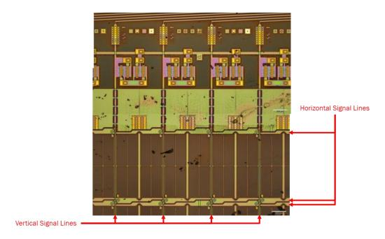
47. As shown below, the surge protection circuit has a plurality of floating-gate field effect transistors, each having a channel capacitance and including a floating gate electrode, a source electrode, and a drain electrode. The source and drain electrodes of the transistors are connected to the vertical signal lines.
