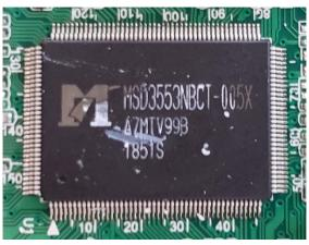
50. Upon information and belief, the MSD3553NBCT-005X controller is expected to have features and components similar (or identical) as other MStar LCD processors, including the MST703 LCD processor. The driving circuit of the MST703 has a gamma compensating circuit in a display controller block, as shown below.
