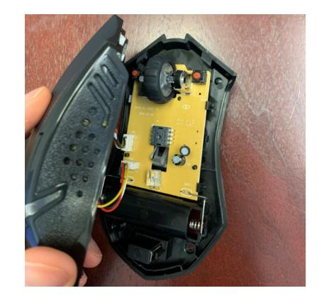
14. The accused products include a an N-stage switch for setting a resolution value, the N-stage switch circuit having a switching button capable of being manually switched to one of positions 1 to N, and accordingly activating a connected resolution setting pin to indicate a state, where N is a positive integer.
