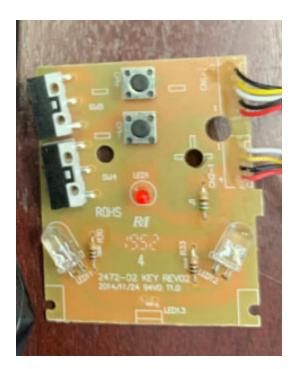
15. The accused products include a mouse micro controller with a register, coupled to the X-Y axis plane displacement detector and the switching circuit, the mouse micro controller determining the resolution value based on the state of the connected resolution setting pins.
