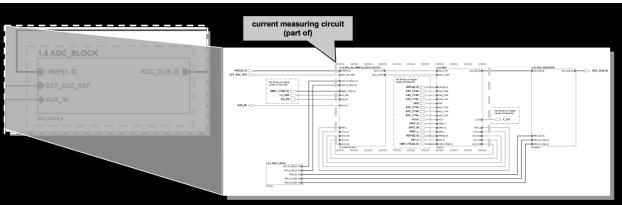
e. said current measuring- and voltage regulating circuit providing to the data conductor a voltage signal which is dependent on a current measuring result and a voltage comparison. For example, the current measuring and voltage regulating circuit described above of the Sony Bravia 55A1 OLED Television provides to the data conductor a voltage signal that is dependent on a current measuring result and a voltage comparison, as shown below.
