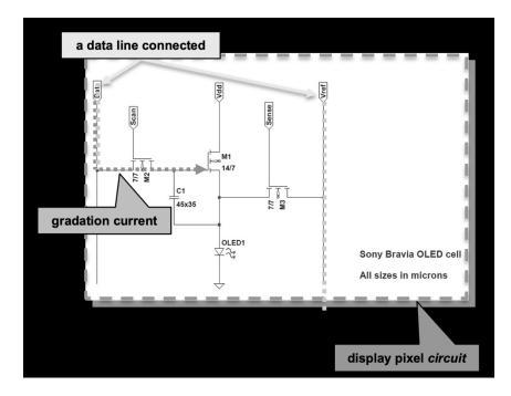
c. a threshold voltage detection circuit which detects a threshold voltage peculiar to the drive element of the display pixel through the data line. For example, the display drive apparatus of the Sony Bravia 55A1 OLED Television comprises a threshold voltage detection circuit that detects a threshold voltage peculiar to the drive element of the display pixel through the data line, as shown below.
