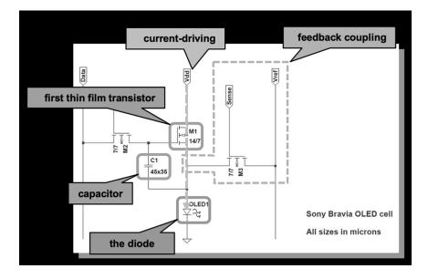
c. a second transistor which is connected by a current-conducting electrode with a gate of said first transistor and by a second current-conducting electrode with a data conductor and by its gate electrode with a scanning signal conductor. For example, the driving circuits of the Sony Bravia 55A1 OLED Television also have a second
