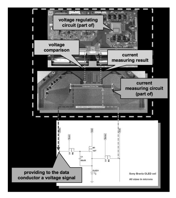
f. so that the diode during driving of said gate of said third transistor due to its non-linear switching characteristic acts as a switch for a current deviation in said current measuring- and voltage regulating circuit. For example, in the Sony Bravia 55A1 OLED Television, the diode, during driving of the third transistor's gate, due to its non-linear switching characteristic, acts as a switch for a current deviation in the current measuring and voltage regulating circuit, as shown below.
