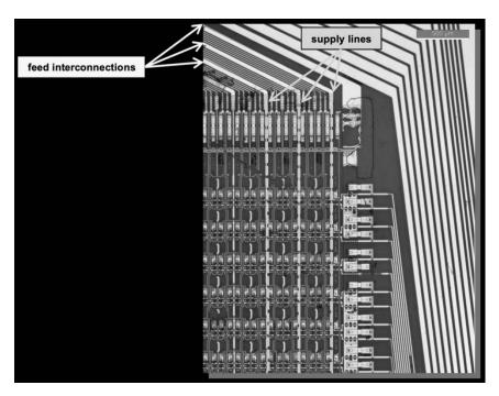
f. a plurality of pixel electrodes each of which is electrically connected to the other of the source and the drain of a corresponding one of said plurality of driving transistors. For example, the display panel of the Sony Bravia 55A1 OLED Television comprises a plurality of pixel electrodes that are electrically connected to the other of the source and the drain of corresponding driving transistors, as shown below.
