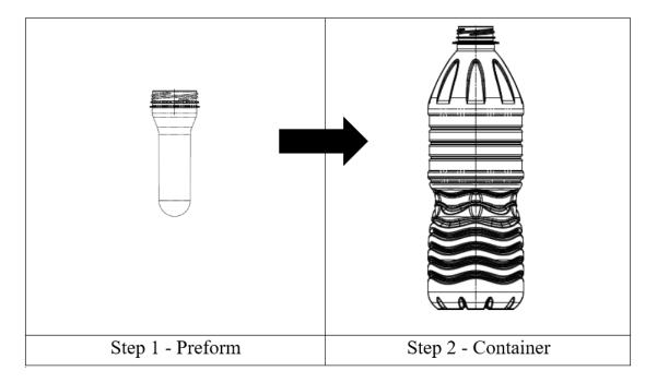
18. In the injection molding process, the neck of a preform is molded into the desired shape of the opening for the final container.
