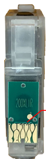
printed circuit board (green) with low voltage electronic device located on back
