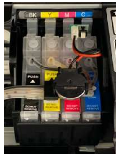
Defendants' Model No. 200XL CISS product installed in the Representative '116 Epson Printer
