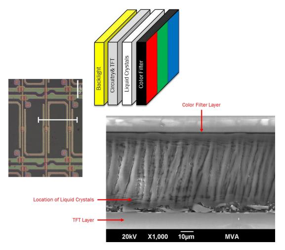
53. As shown below, the TFT array substrate of the HannStar LCD Model No. A4HSN55003093 comprises TFTs.
