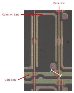
57. The Accused Product has a data line intersecting the gate line with a gate insulating
