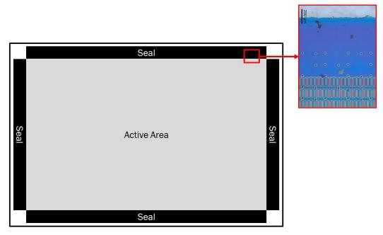
64. The Accused Product shown below has a spacer in the seal to make a gap between the array substrate and the opposing substrate constant.
