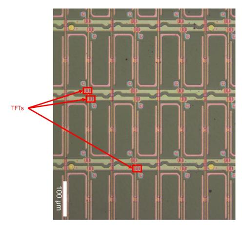
54. The teardown image below shows that the Accused Product has scanning lines on the first substrate, orthogonal signal lines, and a TFT near the intersections of scanning and signal lines.
