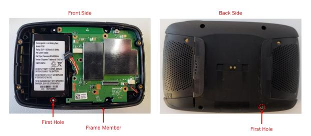
75. The Accused Product has a liquid crystal module with an LCD panel in the front and a frame in the back. The module is mounted to the frame member by way of a threaded screw hole which is in alignment with the hole in the frame.
