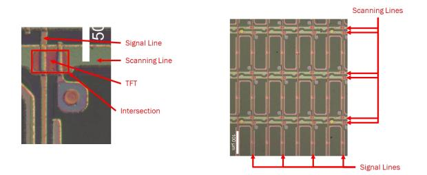
55. Each TFT acts as a switch that operates its respective individual pixel using the circuity lines. In that way, the pixels can be turned on and off to create an image on an LCD by allowing or preventing light to pass through. The individual pixels are more apparent when a color filter layer overlays the circuits as shown in the image below for the HannStar LCD Model No. A4HSN55003093.
