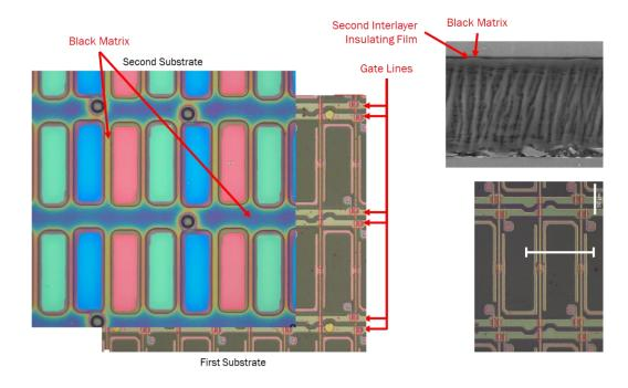
60. The Accused Product shown below has a columnar spacer located above the gate line apart from the intersection of the gate and data lines.
