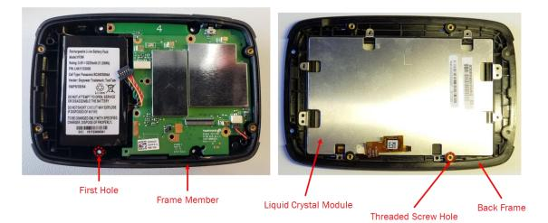
76. There is a screw for attaching the frame member to the liquid crystal module from the back and through the hole in the frame member and the threaded screw hole in the back of the frame of the liquid crystal module.
