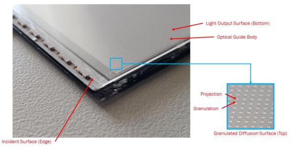
71. The optical guide plate has projections on the granulated diffusion surface with peaks between approximately 10-20 microns, which are higher than the height of the granulations of the granulation diffusion surface, as illustrated below.
