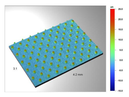
72. The optical guide plate has a reflecting sheet supported by the projections, which forms an air layer between the reflecting sheet and the granulated surface.
