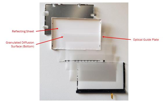
73. As shown below, the optical guide plate has a light source (e.g., an LED strip) opposed to the incident surface.
