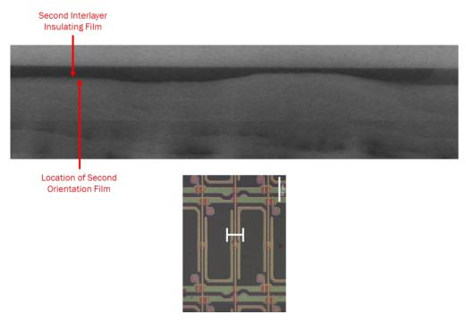
62. As shown below, the columnar spacer is shifted away from a gate line toward a common line.
