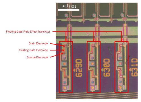
68. In the Accused Product, the transistors respond to surge potentials on the vertical signal lines by turning on and establishing a low-impedance path to ground.
