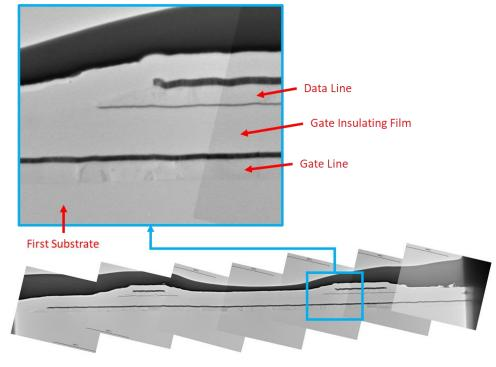
58. The Accused Product also has a first interlayer film coating the data line and a first orientation film coating the first interlayer insulating film, as shown below.
