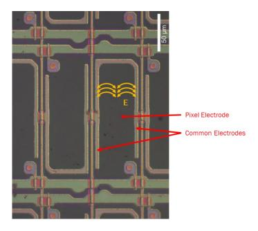
56. Each TFT acts as a switch that operates its respective individual pixel using the circuity lines. In that way, the pixels can be turned on and off to create an image on an LCD by
