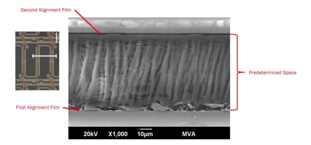
66. The electric field generated by the source and drain electrodes is substantially perpendicular to the non-zero initial alignment angle. Alignment of the first part of the liquid crystal layer does not change when an electric field is generated between the source and drain electrodes.
