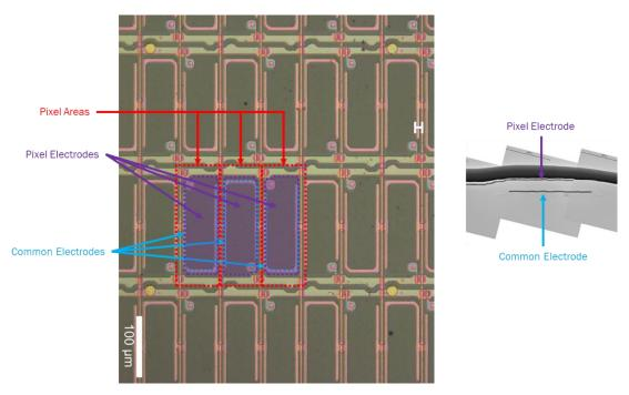
70. The LCD panel of the Accused Product has switching transistors (TFTs) on the TFT array substrate with sources connected to the pixel electrodes, data lines extending outside a periphery of the pixel areas, and gate electrodes extending outside the periphery of the pixel areas.
