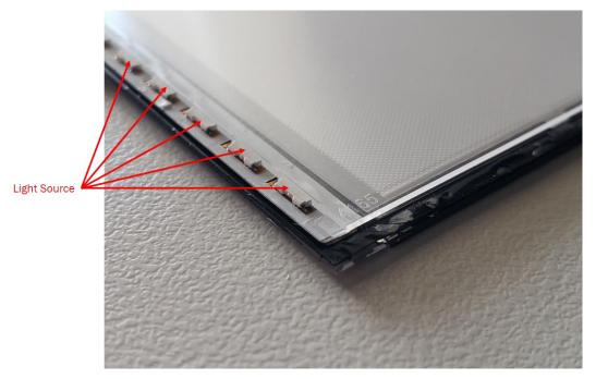
74. The backlight unit has an optical sheet. A transparent reinforcing plate is in contact with a major surface of the optical sheet.
