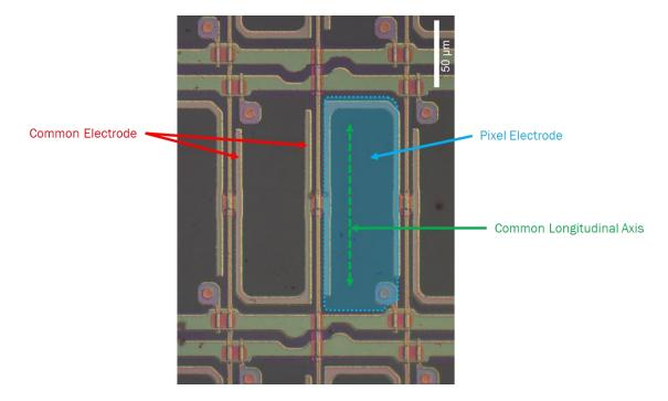
59. The common electrodes in the Accused Product extend substantially parallel to the scanning lines and with comb-tooth projections extending toward the scanning lines. Pixel electrodes are substantially parallel to the comb-tooth projections and located in gaps between comb-tooth projections.
