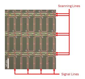
55. The liquid crystal is controlled by an electric field generated by a voltage applied between pixel electrodes and common electrodes on the first substrate.
