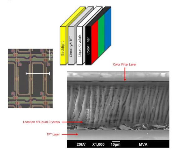
53. As shown above, the TFT-LCD panel contains a TFT array substrate and many TFTs. A teardown image below from the HannStar LCD Model No. A4HSN55003093 shows a sampling of TFTs.
