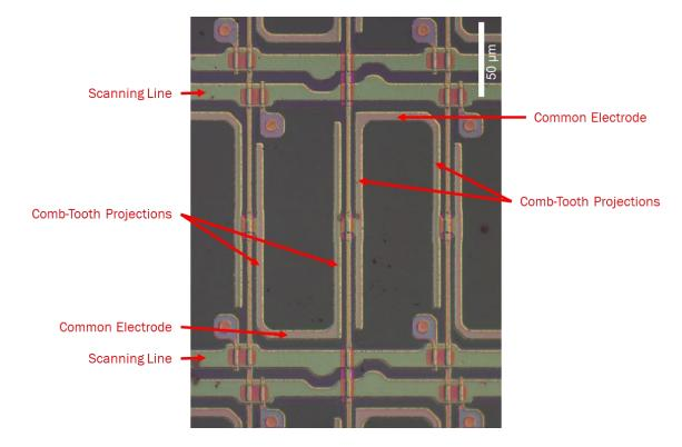
60. In the Accused Product, at least a portion of each pixel electrode is opposite to a common electrode and interposed by an interlayer insulating film.
