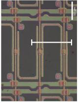
58. The pixel and common electrode have a common longitudinal axis, as shown below, to generate an electric field in the liquid crystal layer parallel to the substrates. The liquid crystal layer has non-zero initial alignment angles relative to the common longitudinal axis.
