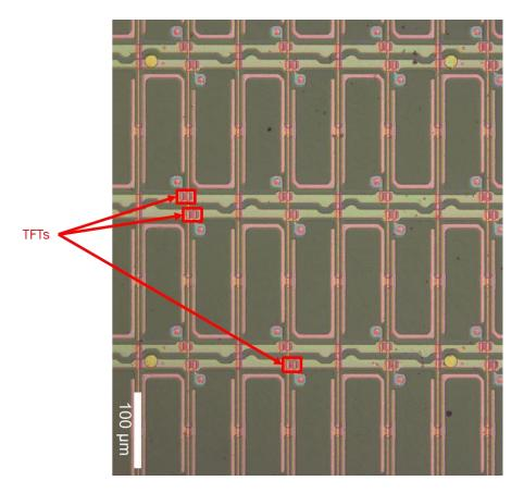
54. As shown above, the TFT-LCD panel contains a TFT array substrate and many TFTs. The teardown image below shows that the Accused Product has scanning lines on the first substrate, orthogonal signal lines, and a TFT near the intersections of scanning and signal lines.
