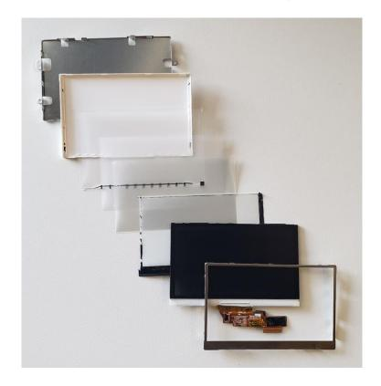
73. The backlight unit has a light source (LEDs), as shown below.
