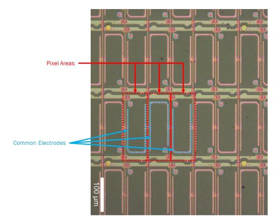
69. As shown below, a pixel electrode for each pixel area is are offset from the common electrode.
