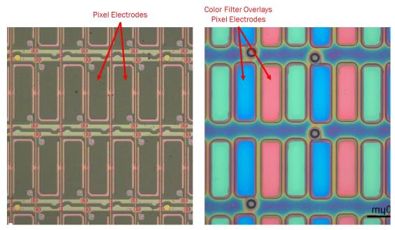
57. The Accused Products have an active matrix type liquid crystal display device with two opposing insulating substrates and liquid crystal in-between, as illustrated below.
