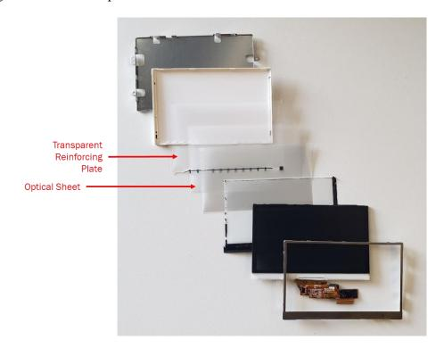
75. The backlight unit has a reflecting member, as shown below. The backlight unit is arranged such that the light source is immediately below the reinforcing plate and between the reflection member and the reinforcing plate.
