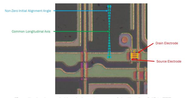
67. For in-plane switching devices, the output of the HannStar LCD's TFTs creates electric fields that orient the liquid crystals to determine whether light passes through the pixels. When an electric field is created, the liquid crystal molecules orient themselves parallel to the
