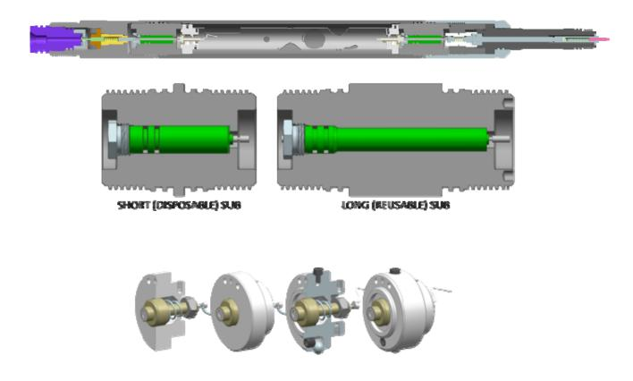
19. The electrical connection assembly in the Thunder Gun either literally or equivalently comprises a tandem seal adapter having a first end, a second end and a bore that extends from the first end to the second end and entirely through the tandem seal adapter. An example of this is shown in the below annotated photo of the Thunder Gun.
