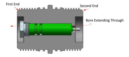
20. The electrical connection assembly in the Thunder Gun either literally or equivalently comprises a perforation gun system comprising a first outer gun carrier, a shaped charge, and a first detonator, wherein the shaped charge and the first detonator are positioned
