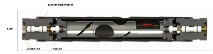
20. The electrical connection assembly in the EZPerf either literally or equivalently comprises a perforation gun system comprising a first outer gun carrier, a shaped charge, and a first detonator, wherein the shaped charge and the first detonator are positioned within the first
