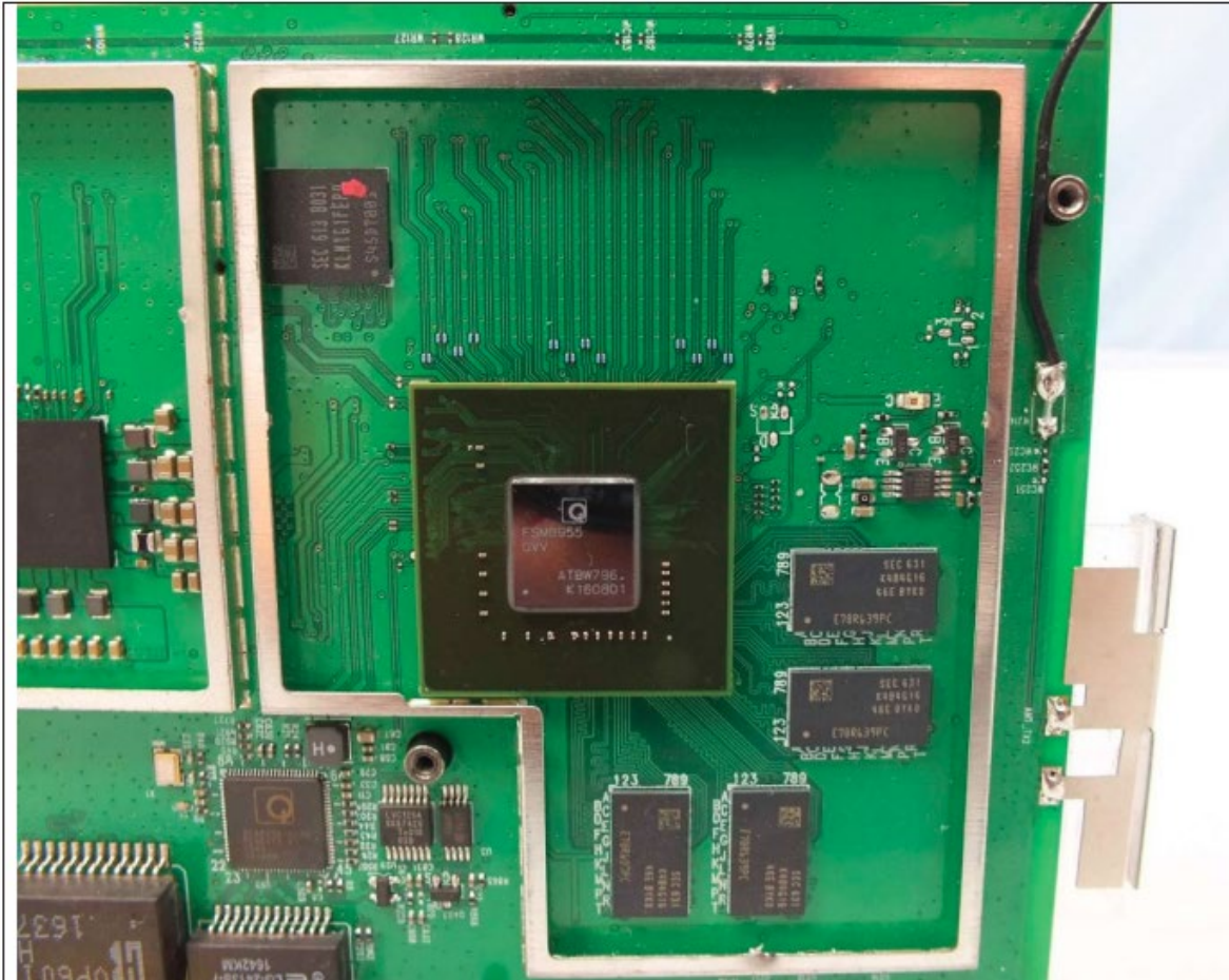
Fig. 12: Illustrating microprocessors used to facilitate data flow (from a tear-down of the T-Mobile 4G LTE CellSpot v2) (FCC ID H7NSS2FII).
