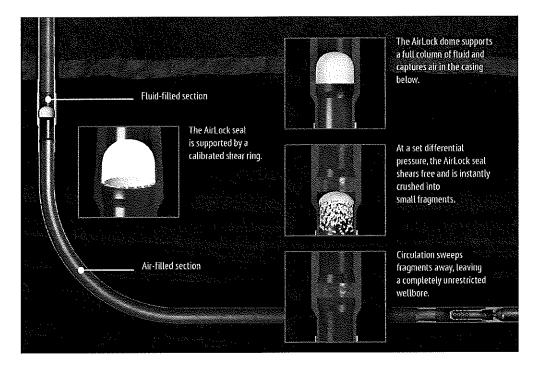
11. The AirLock® system (above in green) is a tubular body attached to the casing string (above in grey). Within the tubular is a rupture disc (above in white). The portion of the casing string above the rupture disc is filled with fluid. The portion of the casing string below the rupture disc is filled with air, which creates buoyancy in the lower portion of the string. This
