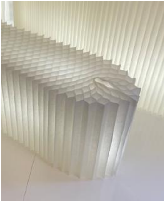
Interconnected Paper Core forming a Cellular Structure in Defendants' Softwall Display
