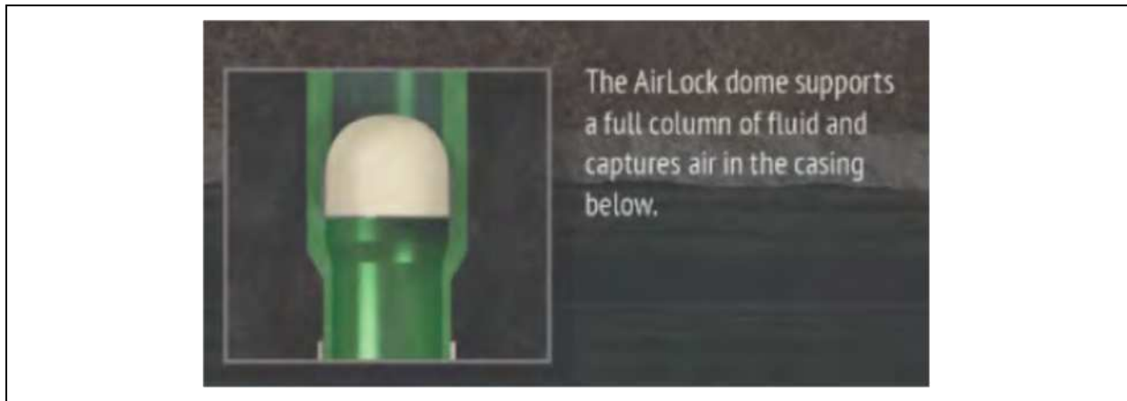
NCS AirLock® Casing Buoyancy System, excerpt of image at paragraph 10 of NCS’s First Amended Complaint
