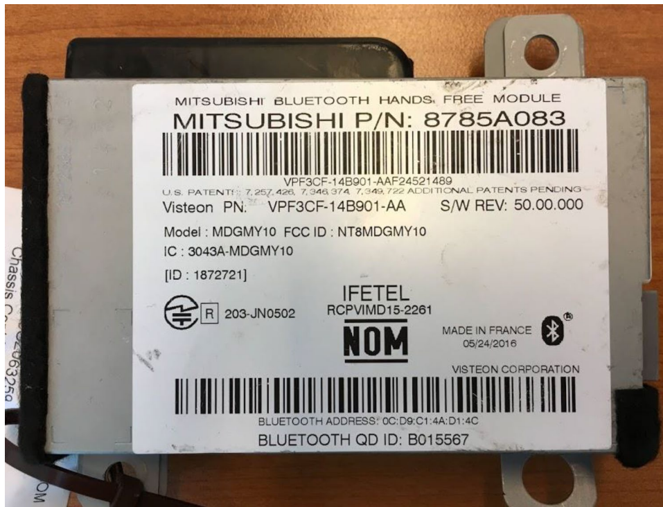
External view of a MELCO MDGMY10 Bluetooth Modul
