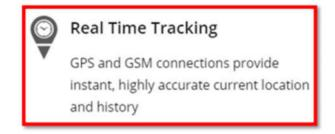
Simply attach your Trackimo to the person or thing you wish to locate and see their location information from the website or mobile app. Device is using GPS satellites and Cellular tower triangulation as second choice to compute the location of the device and report its location via the GSM cellular worldwide network.
