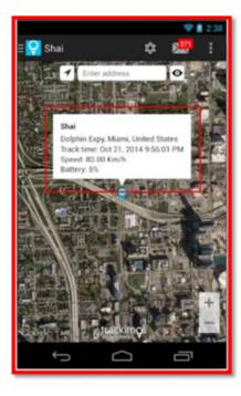
Simply attach your Trackimo to the person or thing you wish to locate and see their location information from the website or mobile app. Device is using GPS satellites and Cellular tower triangulation as second choice to compute the location of the device and report its location via the GSM cellular worldwide network.
