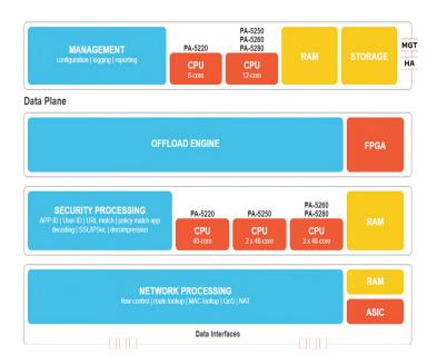
Ex. 18, <a href="https://www.paloaltonetworks.com/resources/pa-series-next-generation-firewalls-hardware-architectures">https://www.paloaltonetworks.com/resources/pa-series-next-generation-firewalls-hardware-architectures</a>.
