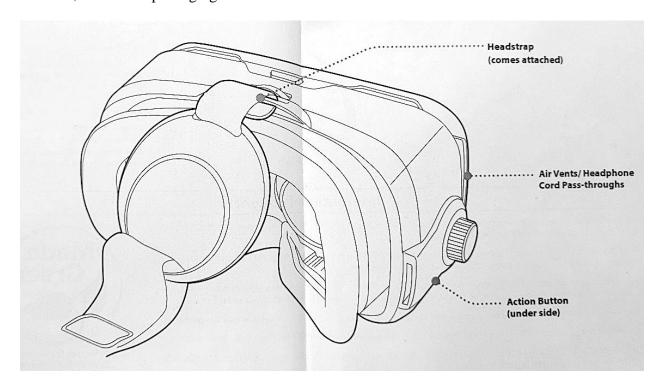
20. The "action button" of the Accused Products, when in a second (or extended) position, contacts the touchscreen of the mobile electronic device within the virtual reality viewer housing.
