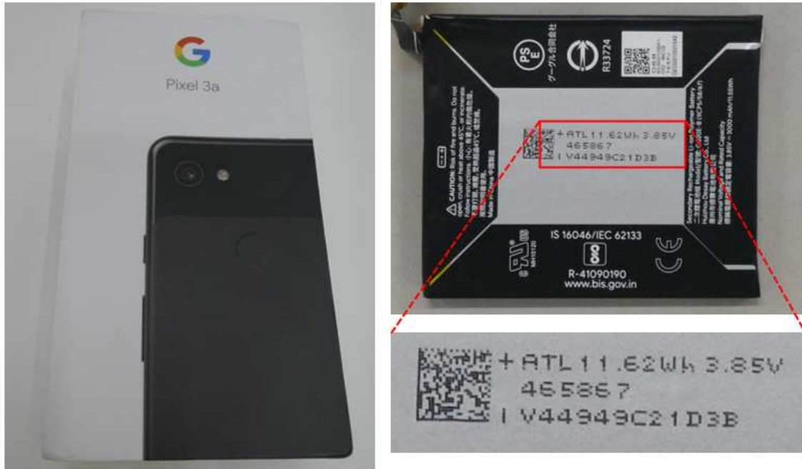
ATL'S LIB Cell No. 465867 in Google Pixel 3a Smartphone
