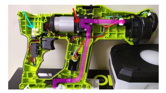
32. The Accused Products include an electrostatic module (red arrow) disposed within the main body housing. An electrode assembly (green arrow) is electrically connected to the electrostatic module via a conductive wire (red wire extending between the red and green arrows).
