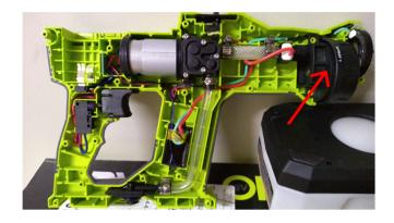
23. The Accused Products have a reservoir configured to have a fluid disposed therein. The reservoir is releasably attachable to the main body housing and is configured to provide fluid to the nozzle assembly when attached to the main body housing.
