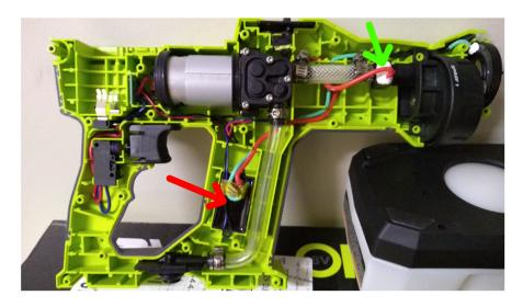
33. The electrode assembly of the Accused Products is configured for electrostatic charging of the fluid. In each of the Accused Products, the electrode assembly includes a conductive ring (red arrow) through which fluid passes en route to the nozzle assembly. The fluid is electrostatically charged via the conductive ring.
