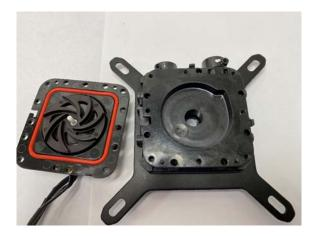
54. The pump chamber of the Exemplary Infringing Products includes "an outlet defined by the impeller cover positioned tangentially to the circumference of the impeller." For example, as the image of the representative Lian Li Galahad product below shows, the pump chamber of the Exemplary Infringing Products has an outlet defined by the impeller cover positioned tangentially to the circumference of the impeller.
