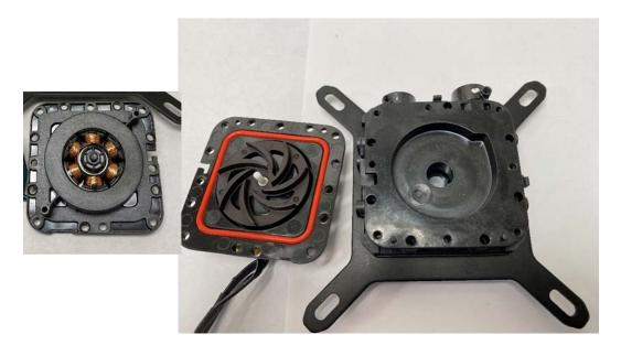
34. The Exemplary Infringing Products further include "a reservoir adapted to pass the cooling liquid therethrough." For example, as the image of the representative Lian Li Galahad product below shows, the Exemplary Infringing Products include a reservoir adapted to pass cooling liquid through it.
