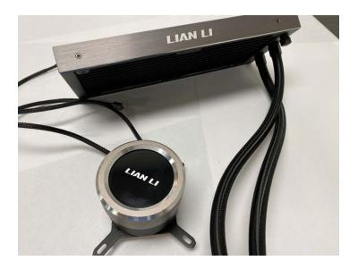
22. The Exemplary Infringing Products further include "a fan adapted to direct air to the heat radiator to dissipate heat from the cooling liquid to the surrounding atmosphere." For example, as the image of the representative Lian Li Galahad product below shows, the Exemplary Infringing Products include a fan that is adapted to direct air to the heat radiator to dissipate heat from the cooling liquid to the surrounding atmosphere.
