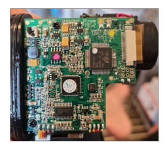
1(b): a signal translator converting differential data signals into a single data signal:—
