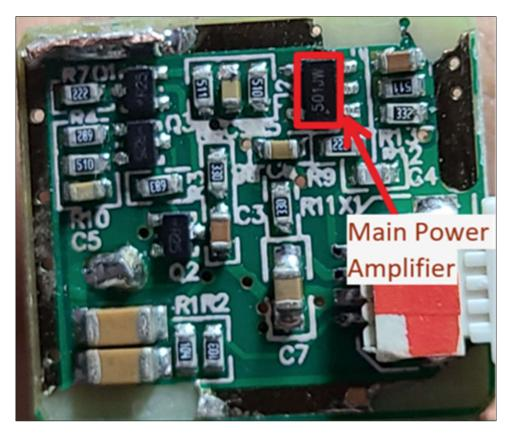
The Main Amplifier amplifies the input voltage of an incoming signal.
