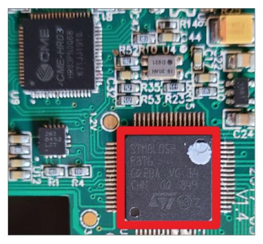
The STM8L052R8T6 contains a reset routine, which outputs a shutdown signal when the input voltage the single data signal is at a high voltage over a predefined ratio.
