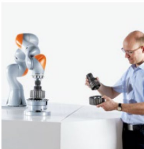
With its integrated torque sensors, the LBR iiwa enables the automation of delicate assembly tasks for force-controlled joining operations and process monitoring.
