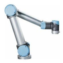
The robot can be programmed to move a tool, and communicate with other machines using electrical signals. It is an arm composed of extruded aluminum tubes and joints. Using our patented programming interface, PolyScope, it is easy to program the robot to move the tool along a desired trajectory.
