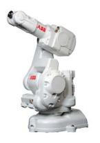
Compact and very powerful. The IRB 140 six axes multipurpose industrial robot handles a payload of 6 kg with a reach of 810 mm (to axis 5) It can be floor mounted, inverted or wall mounted at any angle. The robust design with fully integrated cables adds to the overall flexibility and the collision detection function ensures the robot is reliable and safe.
