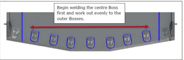
64. This instruction manual (Exhibit L) also states that "[b]oss positioning gauges [shown below] are available for purchase from your local Talon dealer upon request. The Setup Gauge enables easy and accurate positioning of the Talon Boss on the lip plate.":
