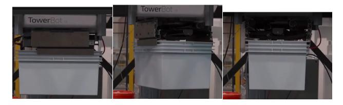
26. URBX also has a Grid Bot that conveys the items from the central voids to the picking stations. One embodiment of the Grid Bot is shown below:
