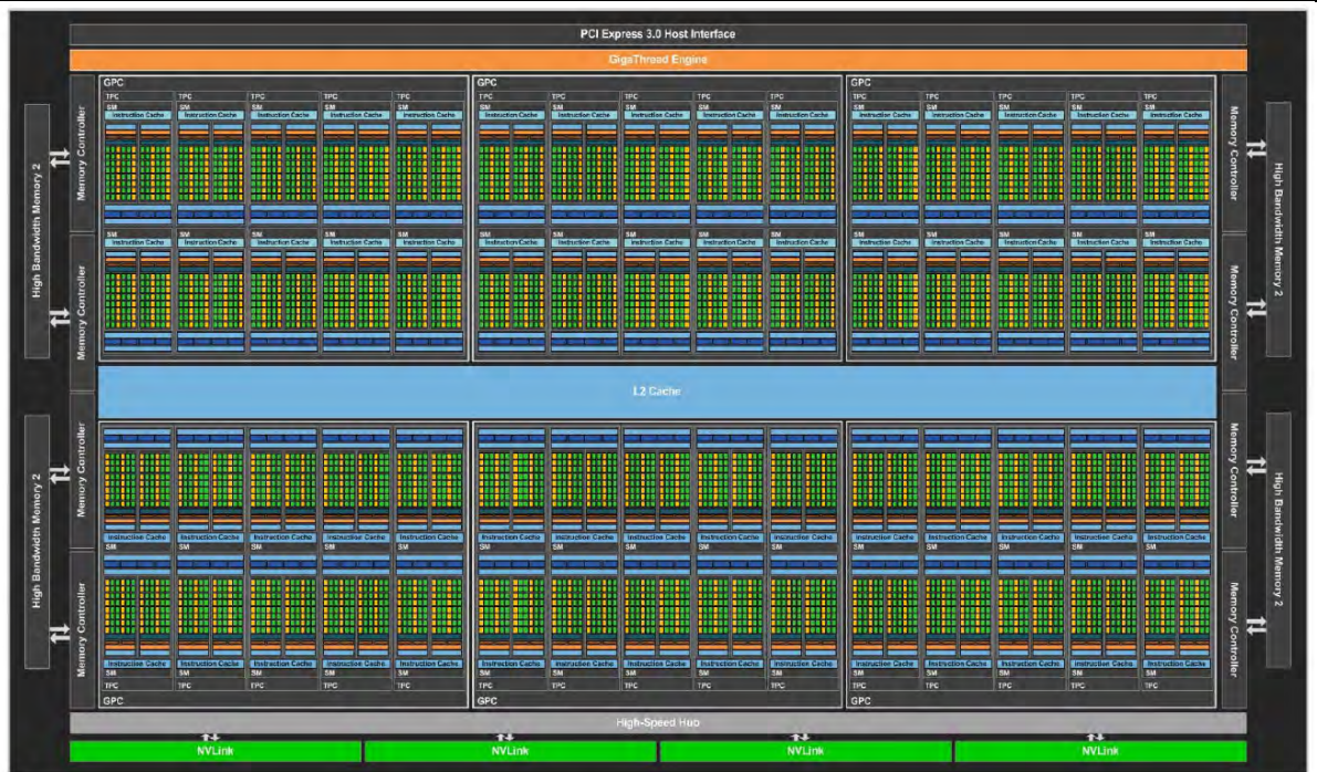
Figure 7. Pascal GP100 Full GPU with 60 SM Units NVIDIA Tesla P100: The Most Advanced Datacenter Accelerator Ever Built Featuring Pascal GP100, the World’s Fastest GPU p. 10, https://images.nvidia.com/content/pdf/tesla/whitepaper/pascal-architecture-whitepaper.pdf
