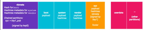
In this setup the xyz partition has a hashtree for integrity-checking. Following the hashtree is a VBMeta struct which contains the hashtree descriptor with hashtree metadata (root hash, salt, offset, etc.) and this struct is signed with key1. Finally, at the end of the partition is a footer which has the offset of the VBMeta struct.
