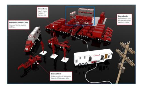
133. Defendants' Electric Frac Operation includes directing the boost fluid to the pump. Specifically, the electric fracturing system developed with Halliburton includes electric pumps coupled to the electric blender via a manifold trailer to direct the boost fluid to the electric pumps.
