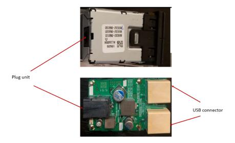
79. Each accused USB charging adapter also includes a power converter that is electrically connected to the plug unit and to at least one USB connector. The power converter can convert a vehicle's DC voltage input at the plug end of the adapter to a 5V DC voltage output at the USB connector for charging a mobile device. The power converter comprises numerous electrical parts on the motherboard, including passive components such as inductors,
