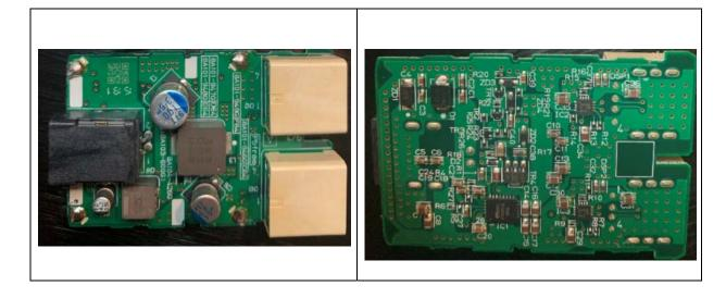
80. Each accused USB charging adapter also includes an identification subsystem electrically connected to the USB connector, including to the D+ and D- pins of the USB connector. The identification subsystem includes at least a USB charging port controller, such as TPS2546 from Texas Instruments or its equivalents. A USB charging adapter with two or more ports or connectors may include two or more USB charge controllers, one for each port, as illustrated below.
