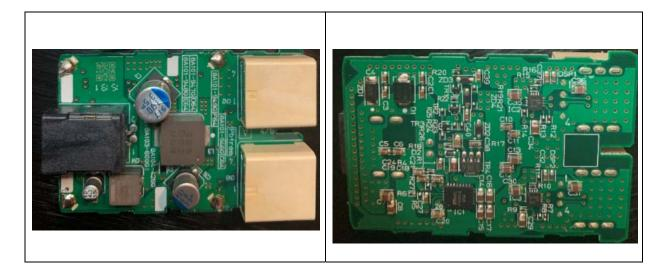
64. Each accused USB charging adapter also includes an identification subsystem electrically connected to the USB connector, including to the D+ and D- pins of the USB connector. The identification subsystem includes at least a USB charging port controller, such as TPS2546 from Texas Instruments or its equivalent. A USB charging adapter with two or more ports or connectors may include two or more USB charge controllers, one for each port, as illustrated below.
