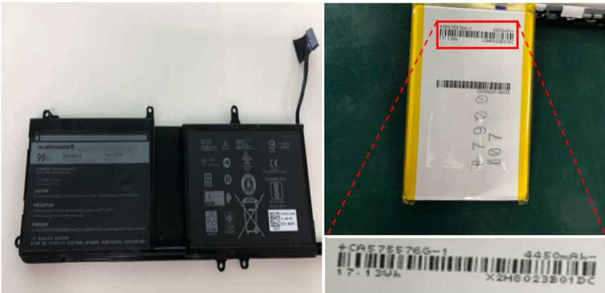
CosMX'S LIB Cell No. CA575576G-1 in Dell d/b/a Alienware 99Wh Type 9NJM1 Notebook Battery
