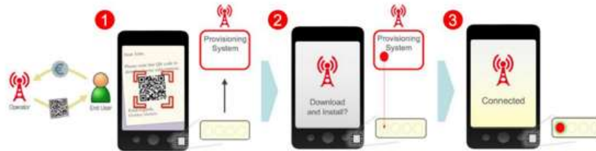
Remote SIM Provisioning Operation – Operator Profile Installation
