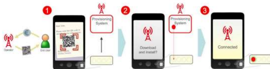
Remote SIM Provisioning Operation – Operator Profile Installation
