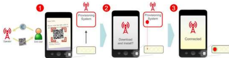
Remote SIM Provisioning Operation – Operator Profile Installation
