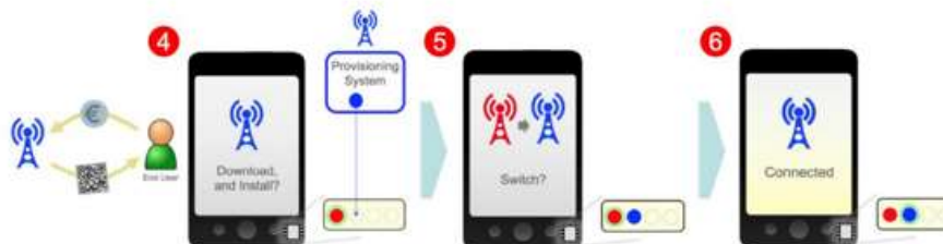
Remote SIM Provisioning Operation – Operator Profile Selection
