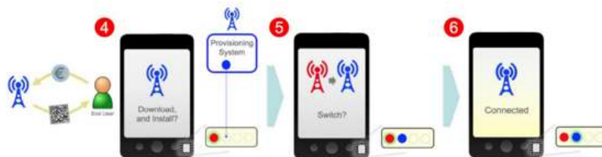
Remote SIM Provisioning Operation – Operator Profile Selection
