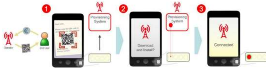
Remote SIM Provisioning Operation – Operator Profile Installation
