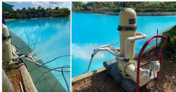
Use of portable exterior filters with localized effect: Not a swimming pool
