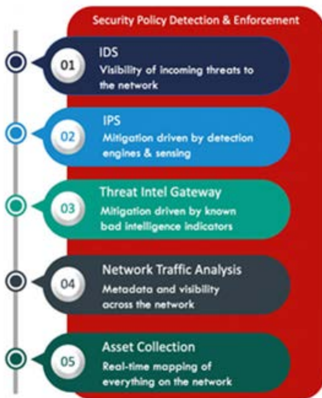
Figure 6c: Policy Controlling Security Detection & Mitigation
